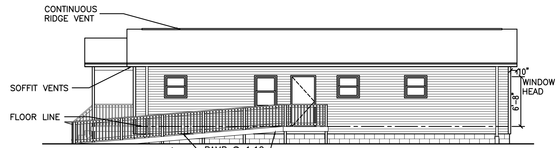
IF RAMP BECOMES LONGER THAN 30' IN LENGTH, PROVIDE INTERMEDIATE 5'-0" x 5'-0" LANDING PER ADA REQUIREMENTS RIGHT ELEVATION - ADA RAMP 1/8" = 1'-0"
